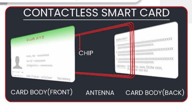
Contactless Membership Smart Cards contain an embedded antenna instead of contact pads attached to the chip for reading and writing information contained in the chip's memory. They do not have to be inserted into a Smart Card Reader. Instead, they need only to be passed within range OR for better security to be placed onto the Smart Card ReaderM/riterto read and store information on the chip.
